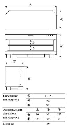
\* The shelf board can be installed at three levels (①,
